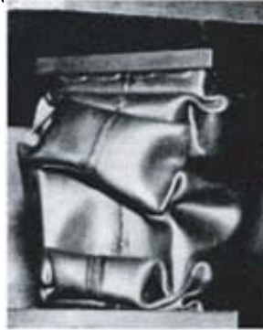
Folding pattern of thin-walled box with very small thickness/width ratio
